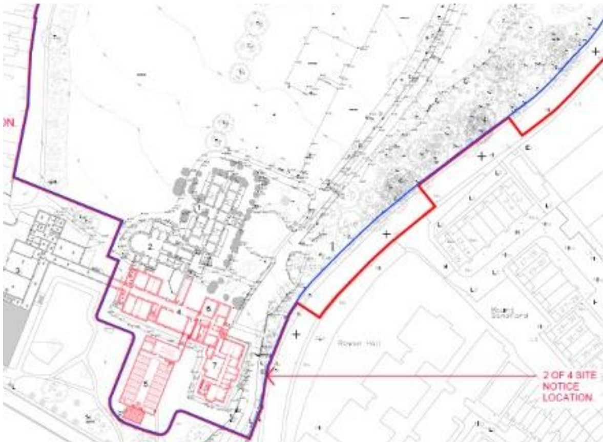
Fig. 72 Proposed identification of building retention and demolition
